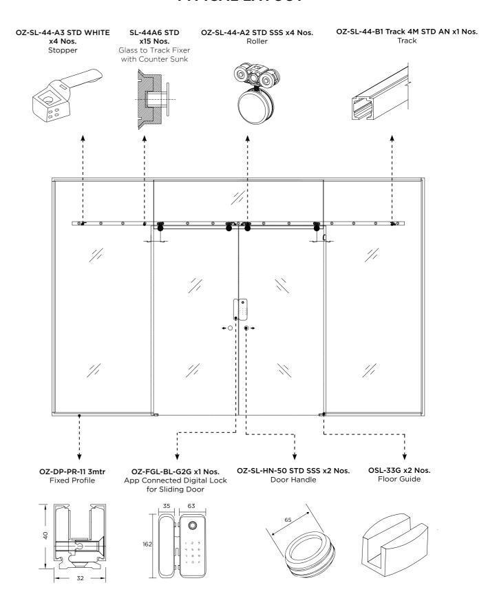
Note: The number of the profiles will change as per the length of the door and according to the site measurement.
