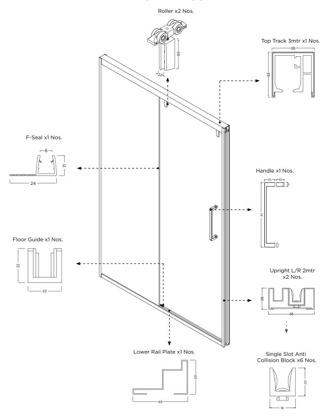
Note: The number of the profiles will change as per the length of the door and according to the site measurement.
