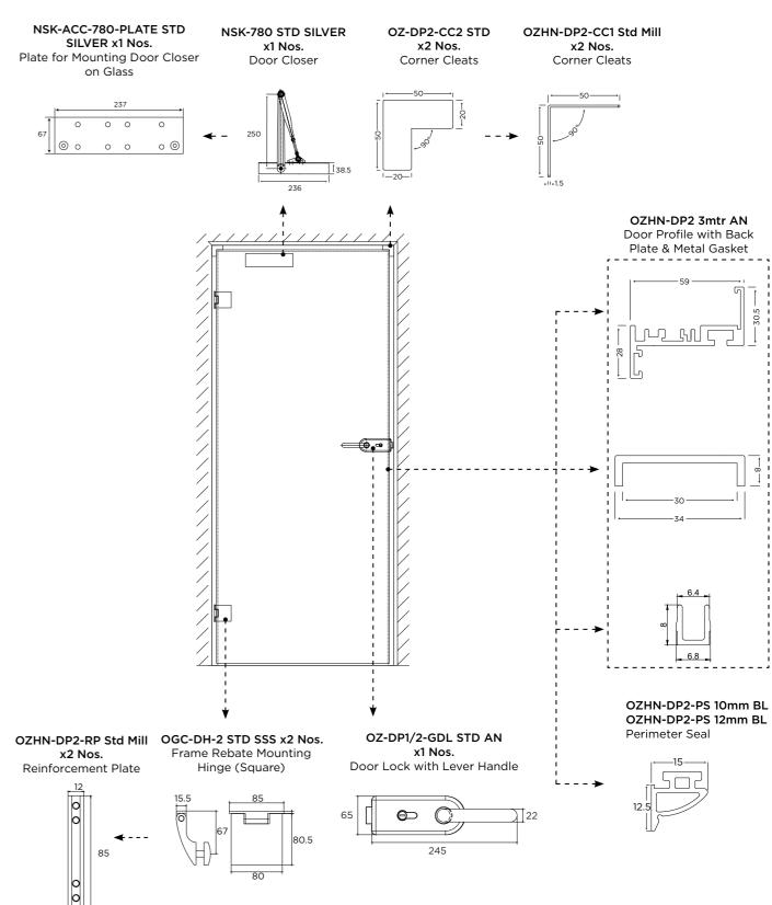
Note: The number of the profiles will change as per the length of the door and according to the site measurement.
