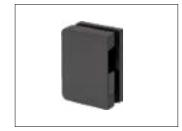
OSDL-11-SB STD BM Strike Box for Offset Glass/Frame to wall Glass Thickness 8-12mm Vertical Adjustment: ±3.5MM Material: ZAMAK Finish: BM
